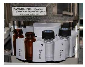
Fig 20.6: Vials of barbiturate solution for assay using gas chromotography
